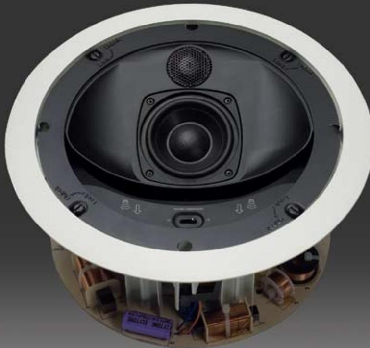
The CS100 is a 3-Way speaker designed for in-ceiling installation. One 8" Copolymer Cone Woofer, a 3-1/2" Neo Copolymer cone midrange and a 1" aluminum dome tweeter are neatly designed into the 12-7/16" diameter frame. The unique design of the CS100 allows for L/R applications, L/C/R and/or surround sound.
