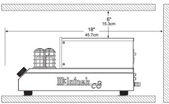
Figure 02- Ventilation requirements
