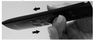
Figure 13- Opening the Remote Control
