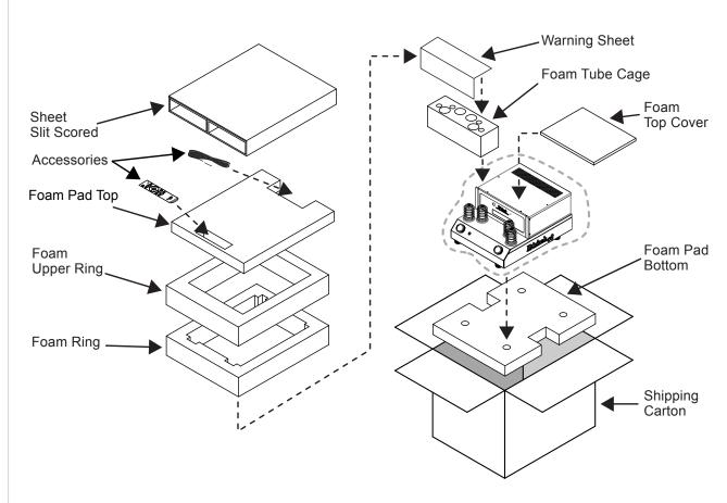
Figure 14- Re-packing diagram
