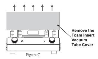
4. Remove from the Foam, the four Vacuum Tube Shield Covers and place them along the side of the C8 Preamplifier. Save the Foam Insert Vacuum Tube Cover with the Shipping Carton for possible future use. Refer to Figure D.
