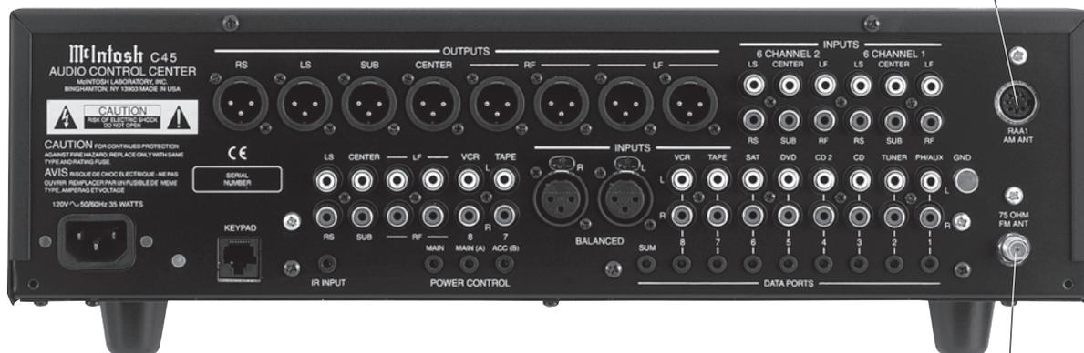
75ohm FM ANT (Antenna) connects to an external FM antenna or cable
