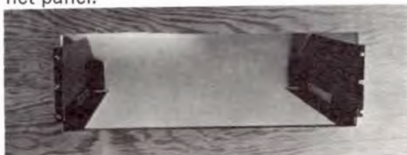
Figure 21. Mounting Brackets installed in cabinet panel.
