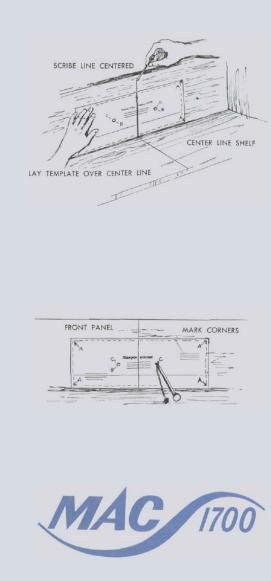
1 On the back of the cabinet panel, scribe a vertical line through the exact center of the area to be cut out.
