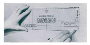
If the cutout is to be located from the front of the panel, begin at 2. If the cutout is to be located from the rear of the panel, begin here.
