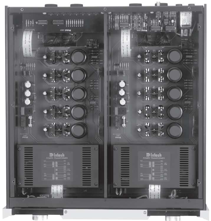
Figure 93 - Top Inside View of the C1000C
