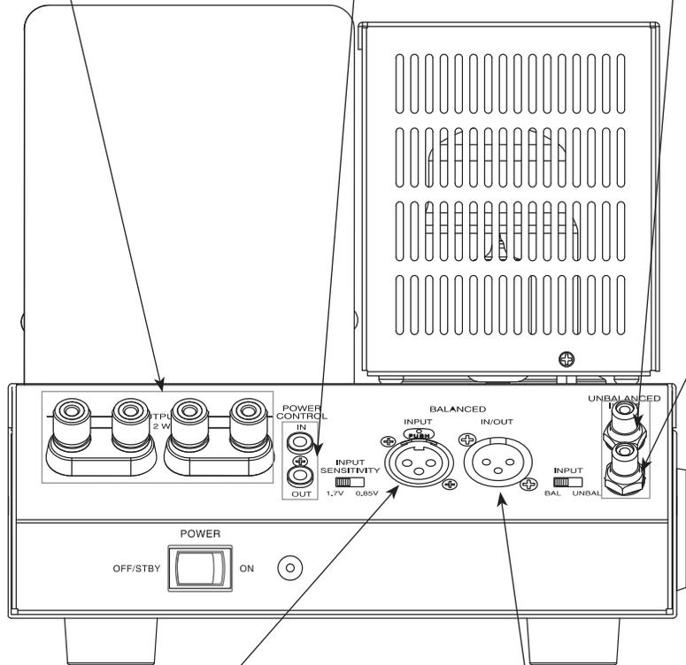
BALANCED INPUT for an audio cable from a Preamplifier or A/V Control Center audio output
