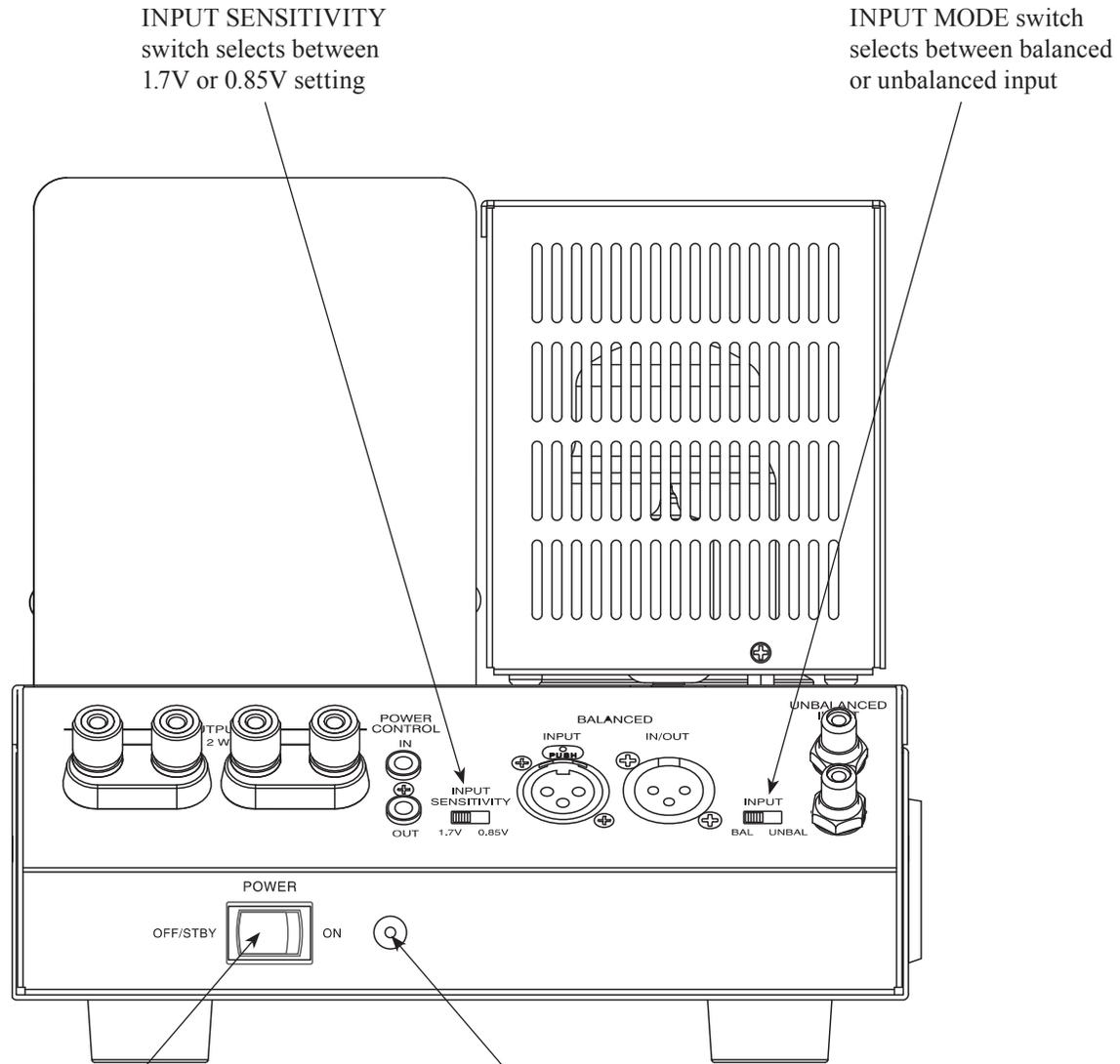
INPUT SENSITIVITY switch selects between 1.7V or 0.85V setting
