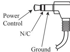
*Note: The Power Control Connecting Cable is available from the McIntosh Parts Department:*
