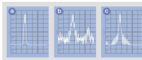
The patented McIntosh Power Guard in the MC58 provides real-time clipping protection without affecting power output or sound quality. **a.** test signal **b.** overdriven amp without Power Guard produces SEVERE clipping **c.** overdriven amp with Power Guard produces NO clipping
