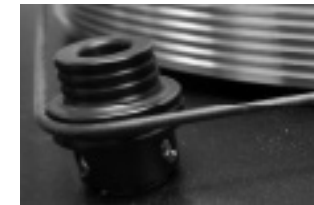
Figure 12– Belt in 45 rpm Position
