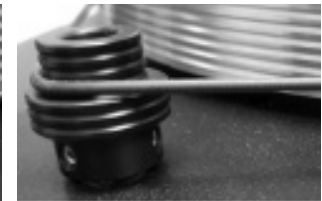
Figure 13– Belt in 33 rpm Position
