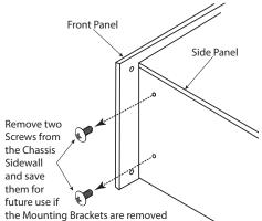
Figure 03- Rack Mount screws
