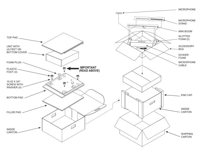
Figure 30- Re-packing diagram
