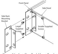
Figure 04- Installing Rack Mount Bracket
