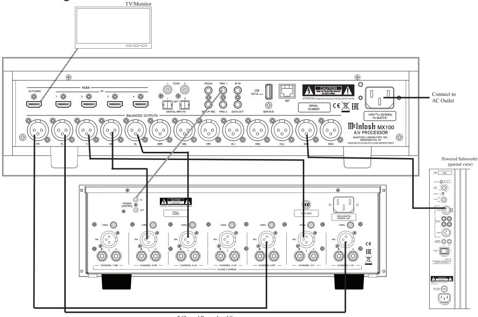
Figure 07– Example 5.1 connection diagram
