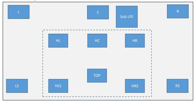
If Dolby Atmos material is played on the above Auro-3D setup, the system will match the speakers, so the LTF/RTF channels are played through the HL/HR speakers and the LTR/RTR channels are played through the HLS/HRS speakers. The HC and TOP speakers will not be used.
