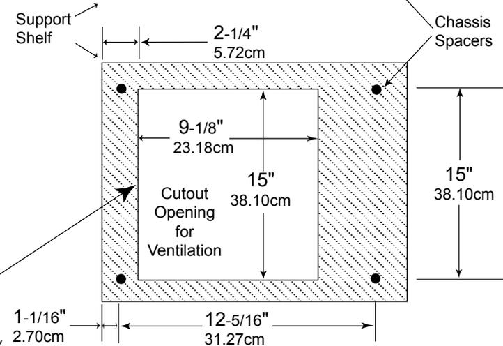
Note: Center the cutout horizontally on the unit. For purposes of clarity, the above illustration is not drawn to scale.
