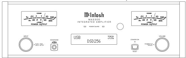
Note: Selection and Adjustment of all Trim Functions may be performed by pressing the Front Panel INPUT Trim Control and then rotating it to select the desired Trim Function. Then use the VOLUME Adjust Control to change the setting. Remote Control TRIM Push-Button together with the LEVEL UP/Down Push-button may also be used. Refer to figures 50
