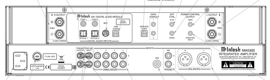
Main Fuse holder, refer to information on the back panel of your MA5300 to determine the correct fuse size and rating
