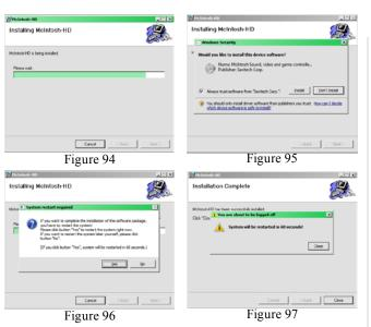
3. When the Windows Security window appears check the Always trust software from "Savitech Corp." box and then the Install button. When the software has been installed, it is necessary to reboot the computer. Refer to figure 96. McIntosh-HD
