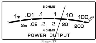
delivered to the Loudspeakers. Refer to figure 77. The meters respond to all the musical information being produced by the Amplifier. They indicate to an accuracy of at least 95% of the power output with only a single cycle of a 2,000Hz tone burst. When an 8 Ohm Loudspeaker is connected to the MC5300, refer to the upper meter scale for power ouput reading. Likewise when a 4 Ohm is connected, refer to the lower meter scale for power ouput reading.
