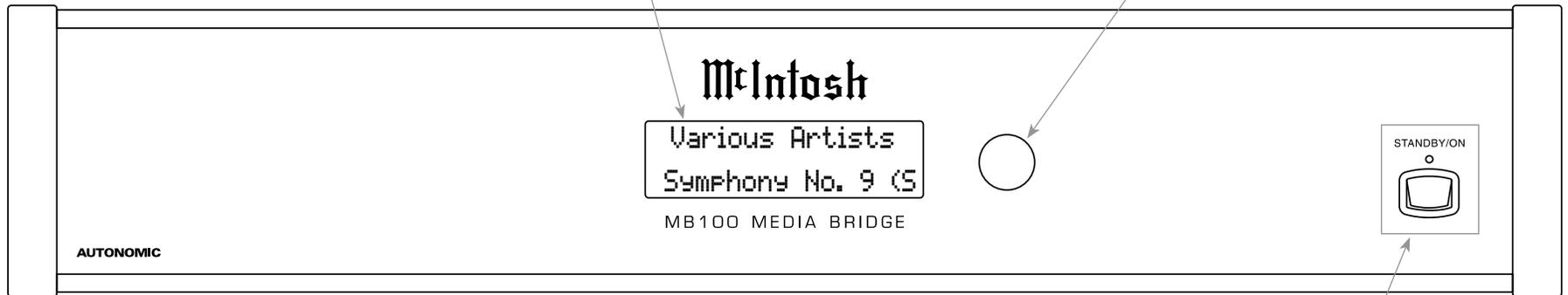
STANDBY/ON Push-button with indicator switches the MB100 ON or OFF (Standby) and resets the microprocessors
