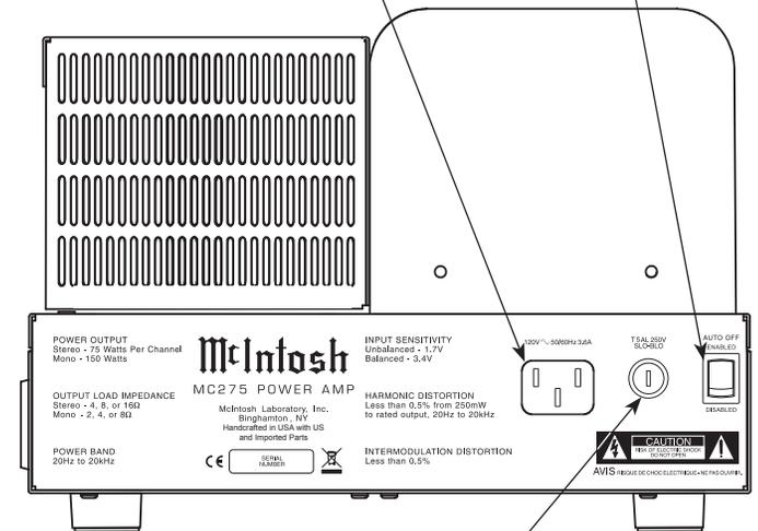
Fuse holder, refer to the nomenclature above this fuse holder to determine the correct the correct fuse size and rating
