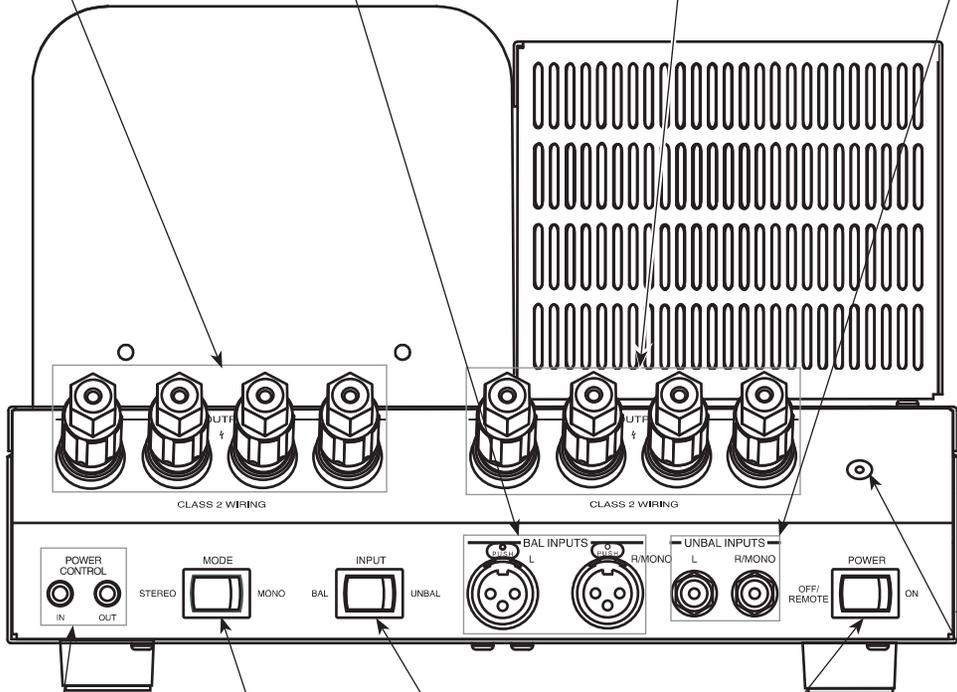
MODE switch selects between STEREO and MONO Parallel modes of operation
