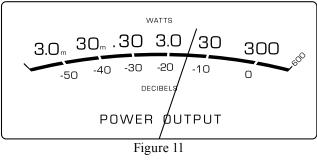
Hold - The meter pointer is locked to the highest power peak in a sequence of peaks. It is electronically held to this power level until a higher power peak passes through the amplifier. The meter pointer will then rise to the newer higher indication. If no further power peaks are reached, the meter pointer will very slowly return to its rest position or lower power level. The decay rate is approximately 6dB per minute.
