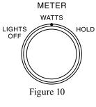
Power Control Input of the MC312 is connected to an Audio Preamplifier or A/V Control Center with Remote Meter Illumination Control, the Meter Illumination will automatically be remotely controlled (On/Off) with the METER Switch set to the WATTS or HOLD position. Watts- The meters respond to all the musical information being produced by the amplifier. They indicate to an accuracy of at least 95% of the power output with only a single cycle of a 2000Hz tone burst.
