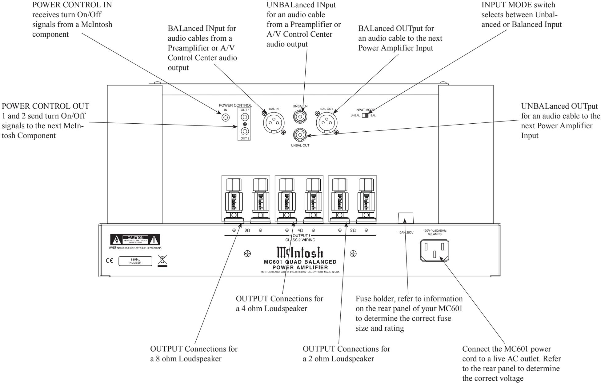
**Caution:** The Loudspeaker ⊖ Negative Connections are above chassis ground. Do not combine any connections together, ground them or connect with another MC601.
