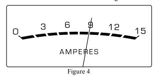
normal for the AMPERES Meter indication to fluctuate especially when a Power Amplifier or Integrated Amplifier is connected to the MPC1500 AC Outlets and music is being played loudly.
