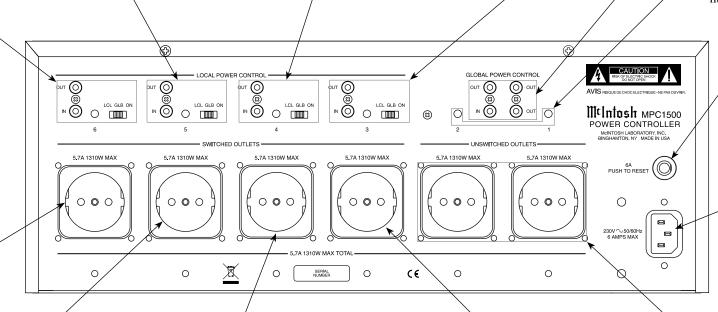
CIRCUIT BREAKER press to reset if the MPC1500 Power Controller will not power up
