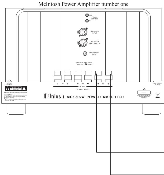
2. Remove all four metal jumpers between Loudspeaker Binding Posts.
