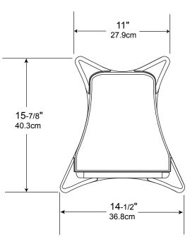
Note: The base is an integral part of the Loudspeaker Enclosure and is not removable for custom installation
