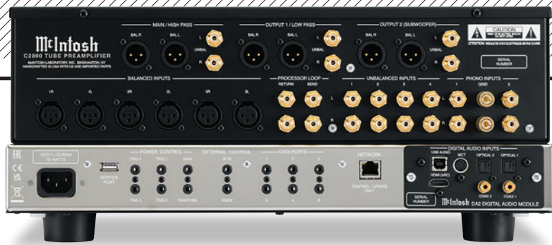
ABOVE: Ethernet is for control only (USB-A as a service port) with digital audio on USB-B (DSD512/384kHz), 2x optical/coax, HDMI ARC and an MCT socket (for DSD). Analogue ins are on RCAs (4x line, MM/MC) and 3x XLRs. A processor loop joins 3x outputs on RCA/XLRs. Multiple trigger and data ports serve automated systems
