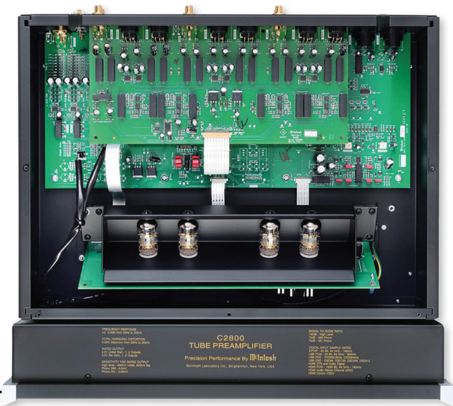
RIGHT: A pair of 12AX7A (ECC83) triodes per channel and one 12AT7 (ECC81) form the core of the line preamplifier while the USB/HDMI/MCT and S/PDIF-equipped DA2 module is housed in a separately screened enclosure, below
