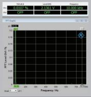
Distortion levels were very low at all frequencies and outputs. There is no crossover distortion: at 10kHz, 1 Watt distortion measured a very low 0.01%, our analysis shows.
