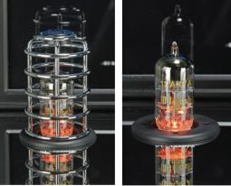
Safety covers over the valves lift off. The bright orange glow comes from underside LEDs, orange indicating warm up or overload.
