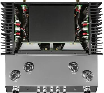
With top cover removed the screened mains transformer can be seen, with power amplifier boards mounted in heatsinks either side. Convention cooling only (no fan) with thermal cutout; ours ran just warm.
