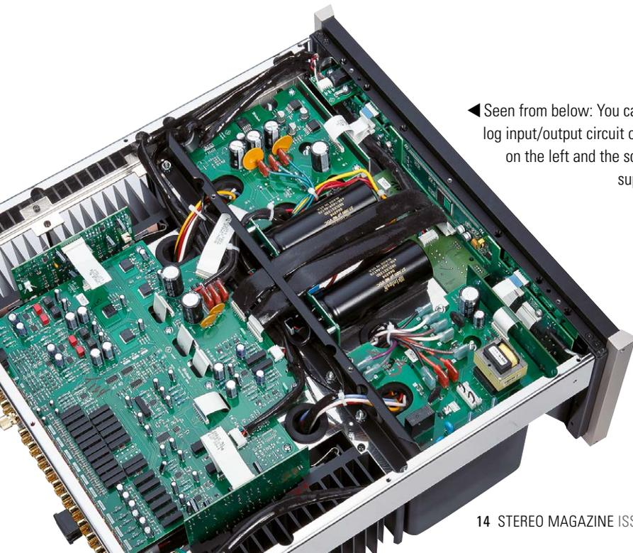
◀ Seen from below: You can see the analog input/output circuit of the McIntosh on the left and the screened power supply to the left.
