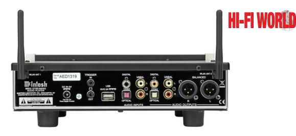
The MB50 has two attenae for a secure wi-fi connection plus balanced and unbalanced analogue outputs as well as a full range of digital in and out connections.
