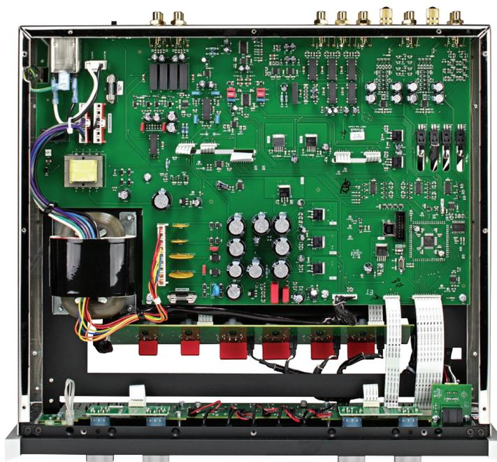
Inside the C70, a big C core mains transformer at left and much solid-state circuitry too.
