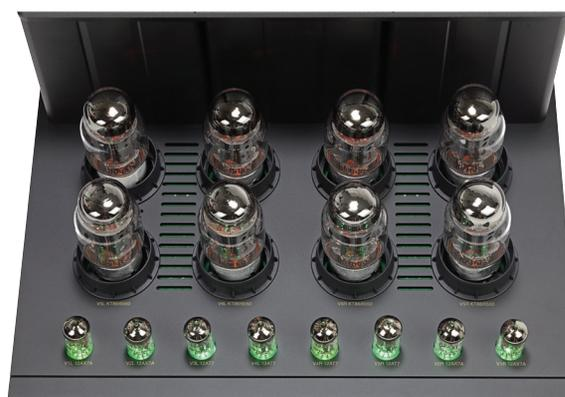
**Eight KT88 output valves, fronted by a row of small signal valves, here lit green by LEDs set beneath them. Blue is a switchable option.**
