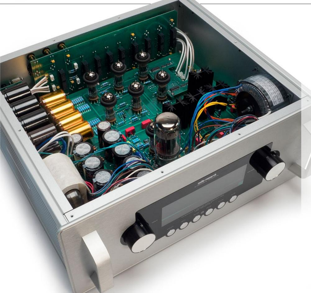
Featuring four inputs, each having the option of single ended RCA or balanced XLR connectors makes the REF 6 one of the most versatile linestages going. Two sets of RCA and XLR variable outputs are joined by a fixed level, record out option – handy for those either stepping up to the tape game or digitizing some of their favorite music. 12 volt trigger and RS-232 interfaces are also available for those wanting to tie everything together, or in a custom install situation.
